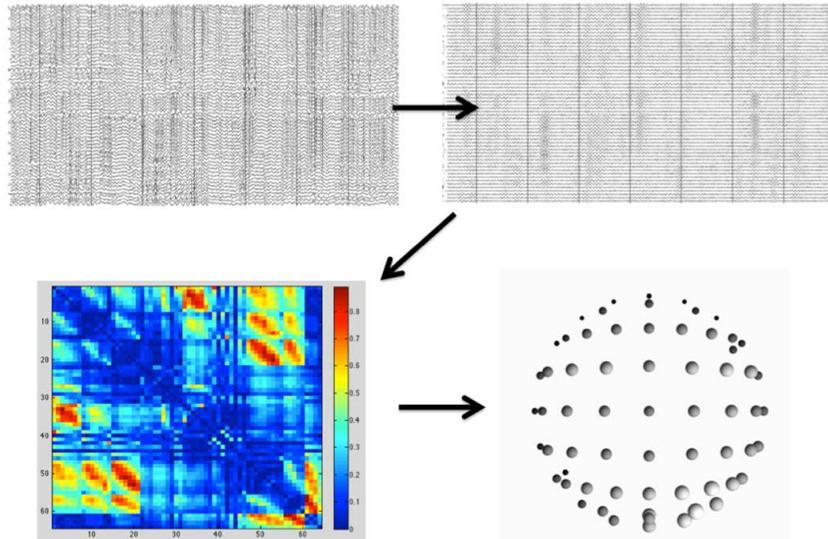
Fig. 1. A schematic view of the feature extraction procedure is represented. Panels respectively represent: raw EEG signals (upper left), band-pass filtered EEG signals (upper right), connectivity matrix containing PLI values (lower left) and role of each node in the network, where the size and colour of each node represent the importance of the nodes (lower right). The EC values were used as feature vectors.
