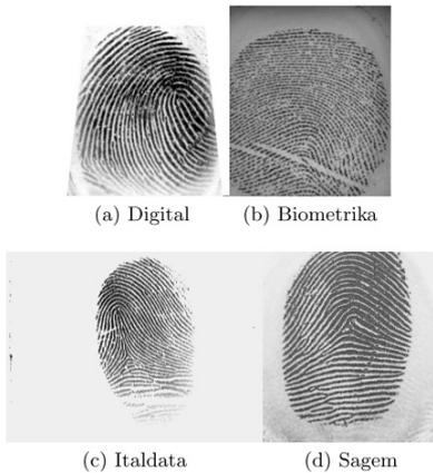
**Figure 2: Examples of fake fingerprint acquired with the 4 sensors.**
