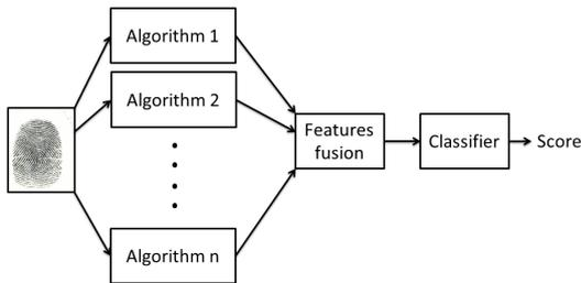
**Figure 4: The fingerprint liveness detection system adopted in this paper.**
