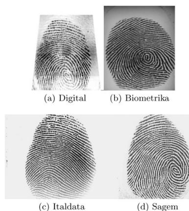
Figure 1: Examples of live fingerprints acquired with the 4 sensors.
