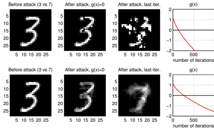
**Fig. 3.** Illustration of the gradient attack on the digit data, for  $\lambda = 0$  (**top row**) and  $\lambda = 10$  (**bottom row**). Without a mimicry component ( $\lambda = 0$ ) gradient descent quickly decreases  $g$  but the resulting attack image does not resemble a “7”. In contrast, the attack minimizes  $g$  slower when mimicry is applied ( $\lambda = 10$ ) but the final attack image closely resembles a mixture between “3” and “7”, as the term “mimicry” suggests.
